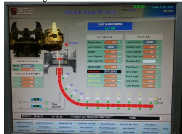
Gambar 3.11 Tampilan Human Machine Interface pada Mesin Continuous Casting
